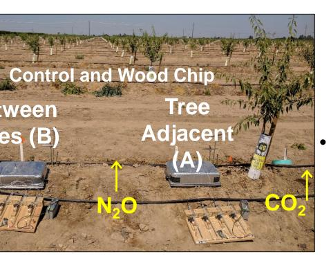
Fig. 4 static flux chambers have three *locations: adjacent (A) and between trees* (B), and in the alleyway.
