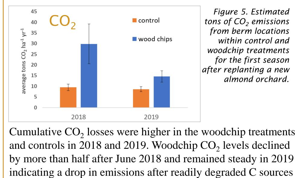
indicating a drop in emissions after readily degraded C sources were diminished. Higher  $CO_2$  rates are consistent with higher levels of microbial biomass and activity associated with organic matter turnover as observed in other recent WOR trials.
